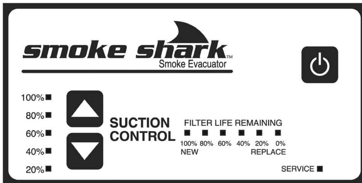
Figure 1 - Control Key Pad
